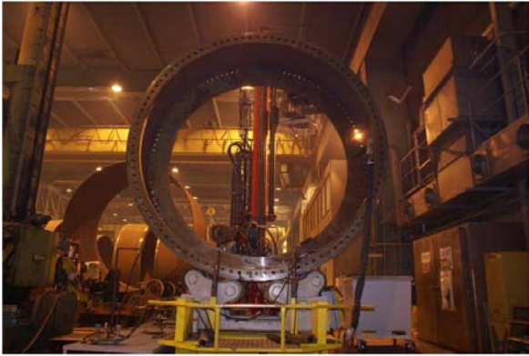
Figure 7. The tower shells' flanges are welded using tandem submerged arc welding (source: Levator Oy).
