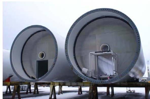
Figure 6. Painted tower sections in different stages of internal installation (source: Levator Oy).
