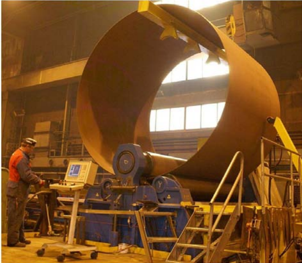
Figure 3. The rolling of the tower shell requires careful work (source: Levator Oy).
